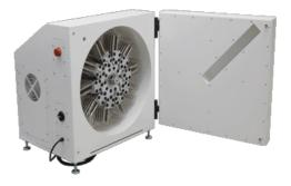
Centrifugal Partition Chromatography (CPC) stands as aunique and innovative chromatographic technique, offering distinct advantages over traditional methods. CPC replaces conventional chromatographic columns with interconnected cells filled with the liquid stationary phase.
